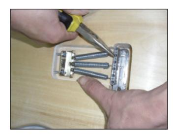
Turn the guitar over and screw the spring claw part-way into the pre-drilled holes at the forward edge of the rear body cavity.
