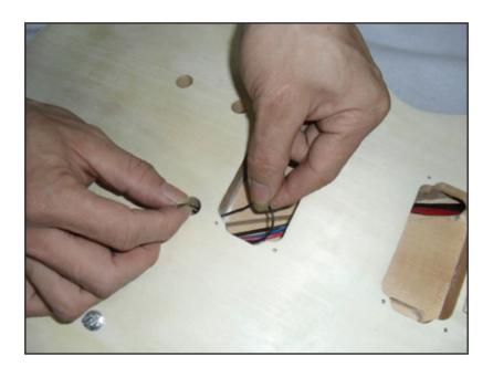
Lead the cables of the pickups from the pickup cavity through the channel to the control cavity and connect them to the potentiometers accordingly.
