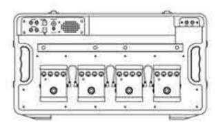
Connect the effects pedals with the 6 pin parallel DC cable. Connect the L-shaped plug to DC OUT.
