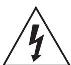
This symbol is intended to alert the user to the presence of uninsulated “dangerous voltage” within the product’s enclosure that may be of sufficient magnitude to constitute a risk of electric shock to persons.
