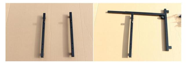
Start by laying out your 2 feet pictured on the left, then attach one of the upright bars to the foot using the small thumb screws (with the large plastic knob) we have 2 types, this is the one with the smallest thread on it.
