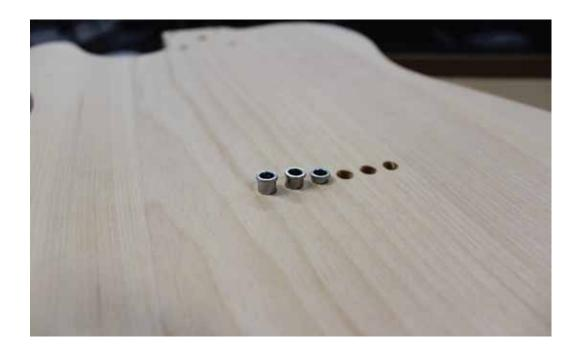
Fitting strings to the guitar is achieved by threading from the hollow screw and the hole, emerging through the relevant saddle on the bridge. Start with the thinnest string in the uppermost position on the bridge.
