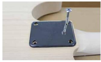
Turn the assembly over and position the neck plate (with its black protective seal) over the four bolt holes at the rear of the body and drive in the four long screws through the neck plate, body and pilot holes in the neck until all fits tightly
